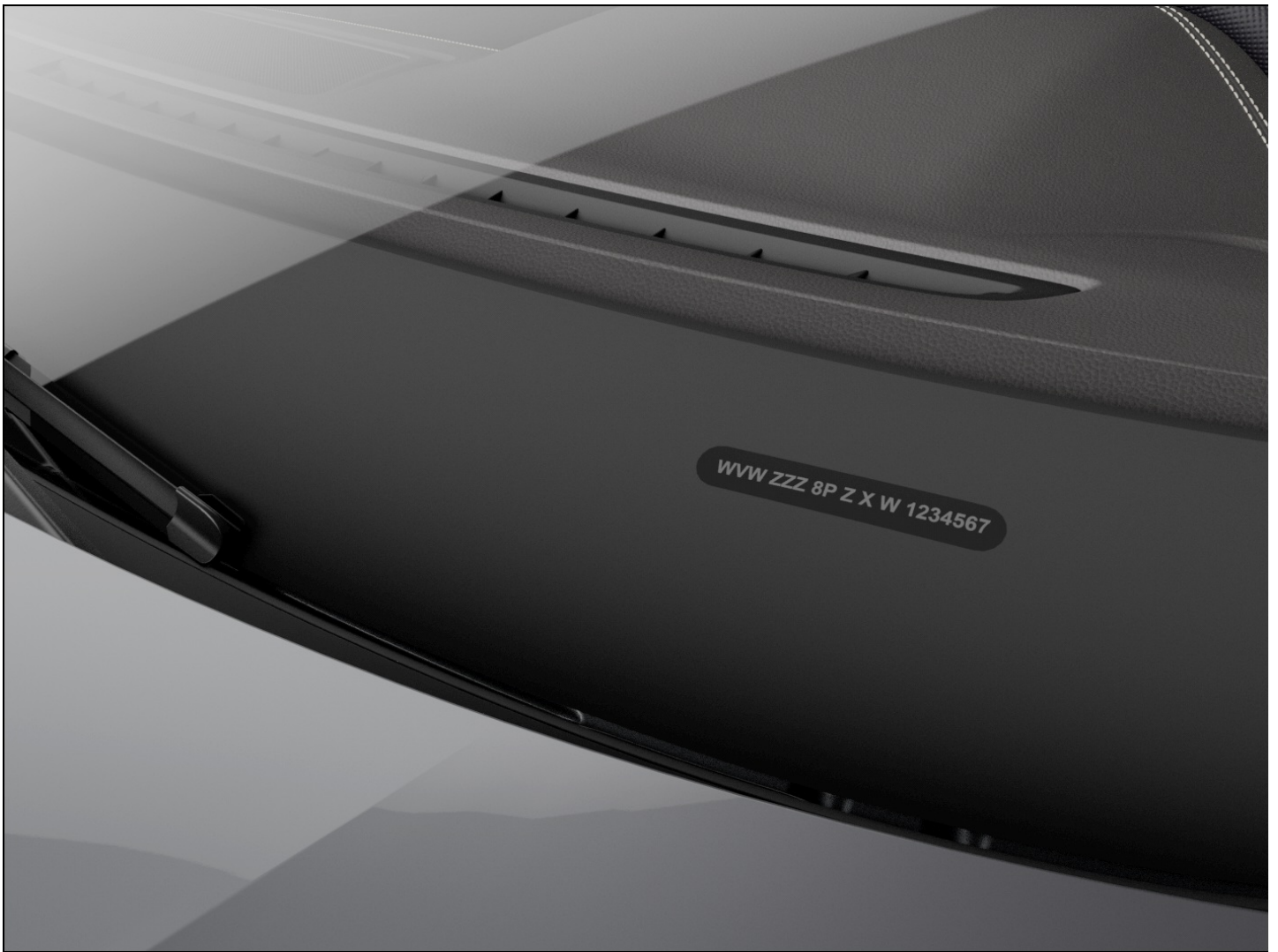
Fig. 184 In the windshield: vehicle identification number (VIN)
