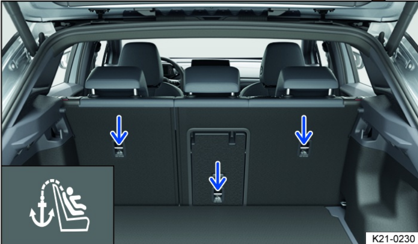
Fig. 31 On the rear side of the rear bench seat: Top tether anchorages for the top tether safety belt.
