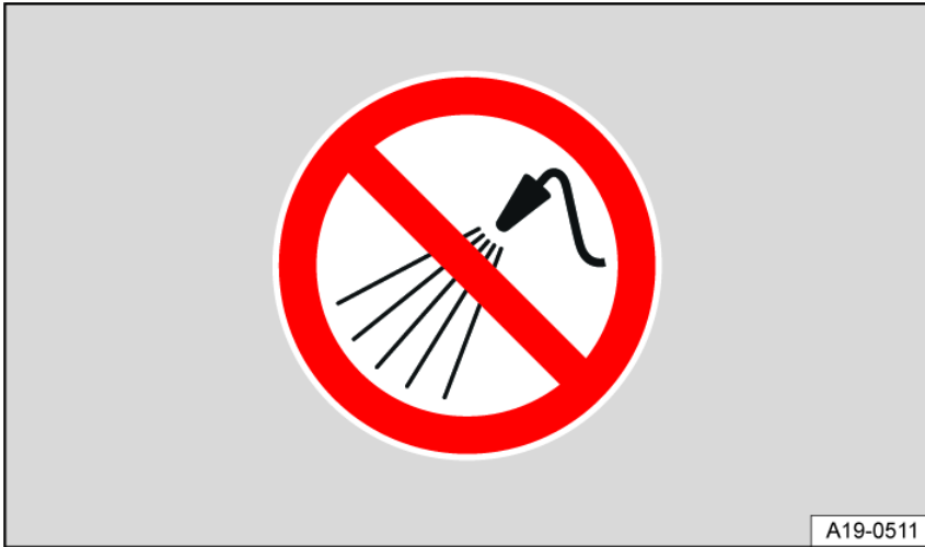
Fig. 178 Warning sign: Do not use pressure washers in the marked area.
