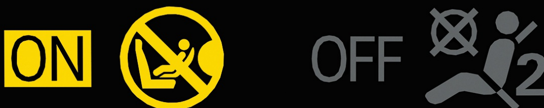
Fig. 22 In the roof console: Indicator light (general example) for the activated front passenger's front airbag.
