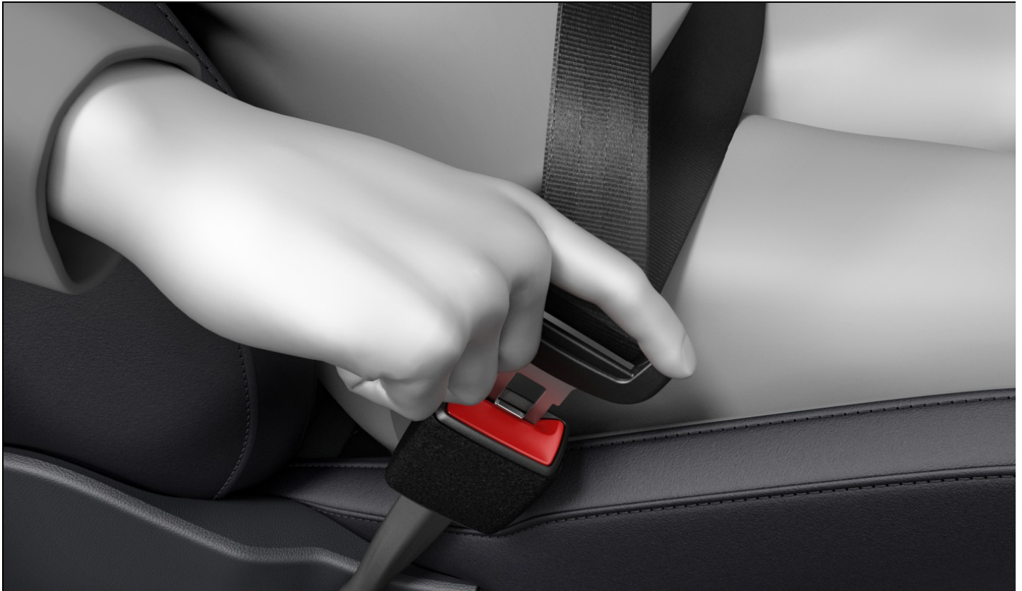
Fig. 16 Inserting the buckle tongue into the safety belt buckle.
