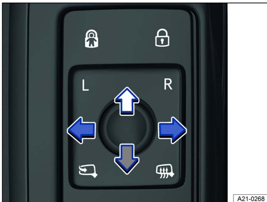
Fig. 79 In the driver door: knob for the outside mirrors.
