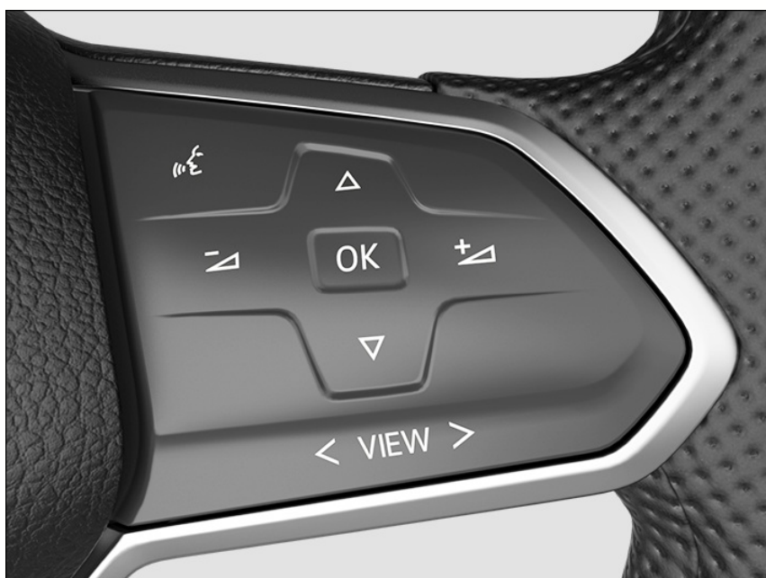
Fig. 9 Right side of the multi-function steering wheel: operating the Volkswagen Digital Cockpit.
