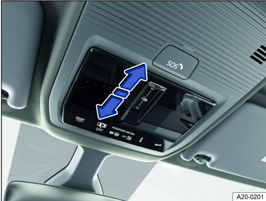
Fig. 81 In the headliner: Function keys for controlling the sunshade.
