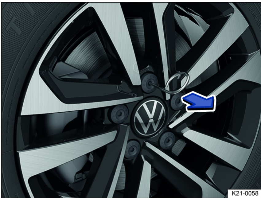
Fig. 169 Remove the caps from the wheel bolts.
