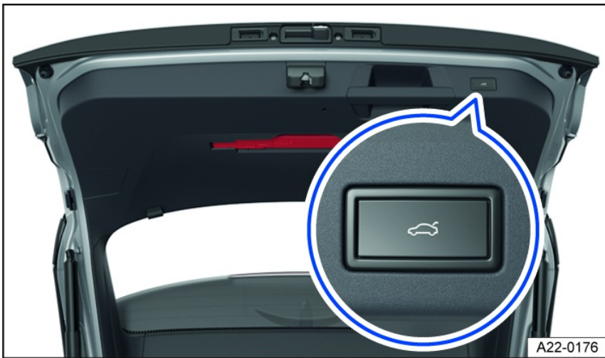
Fig. 53 In the open trunk lid: Button for power closing the trunk lid (general example).
