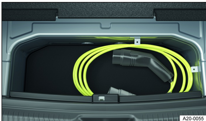
Fig. 137 Under the luggage compartment floor: Storage compartment for the charging cable (general example).
