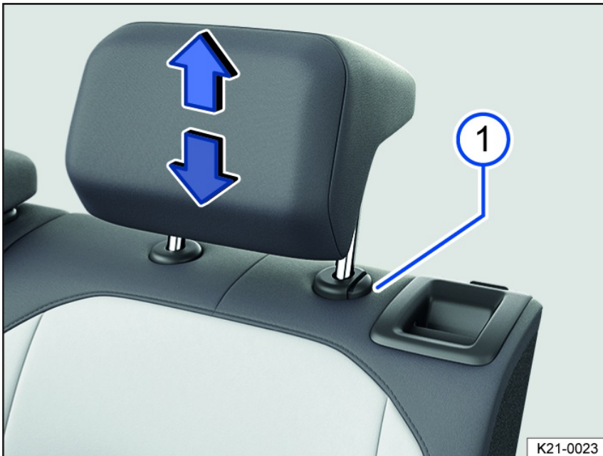
Fig. 66 Removing the rear head restraint (general example).
