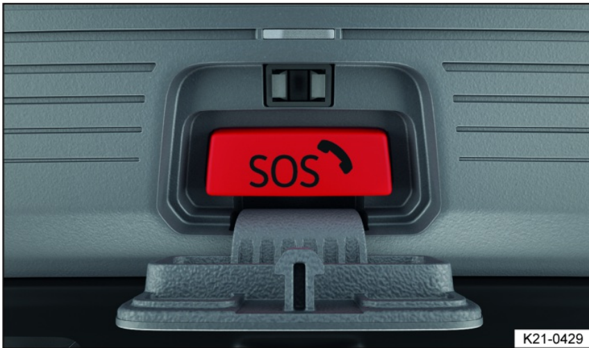
Fig. 37 Located on the roof console: Emergency Call Service button.
