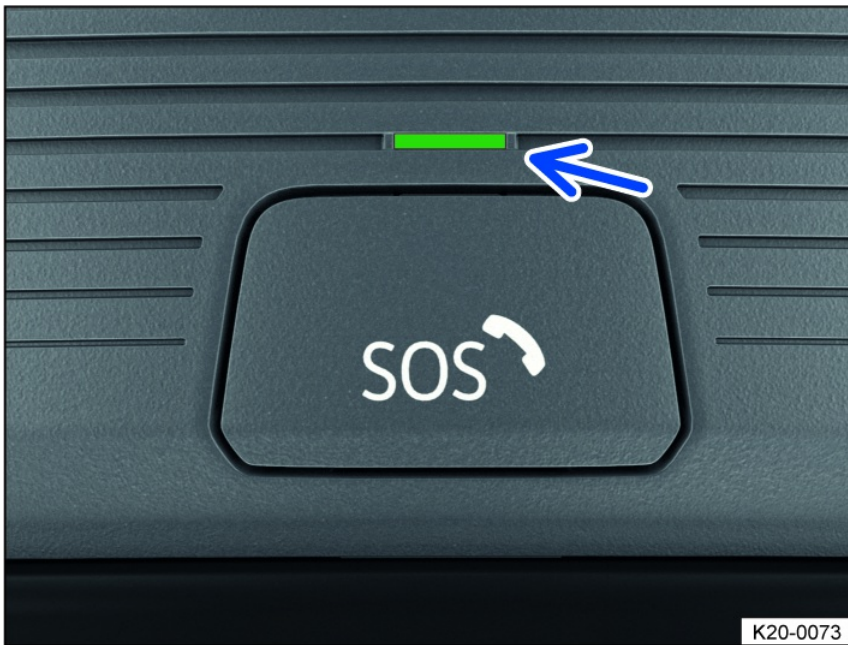
Fig. 36 Located on the roof console: Emergency Call Service button (behind a button cover) and indicator light.
