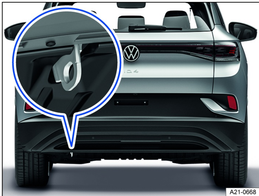
Fig. 155 At the rear of the vehicle: pulling eye for tow truck installation location.
