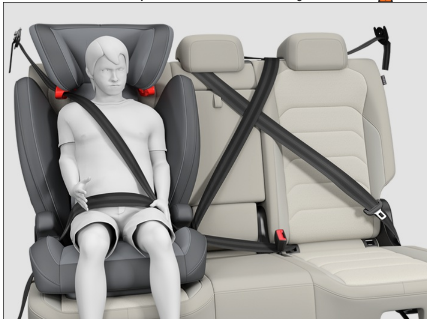
Fig. 34 Correctly fastened child on a booster seat.
