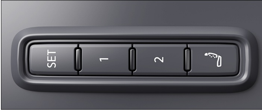
Fig. 69 On the outer side of the driver's seat: memory buttons.
