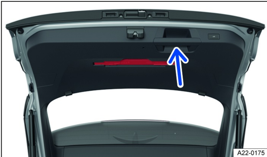
Fig. 51 In the open trunk lid: handle for closing the trunk lid (general example).
