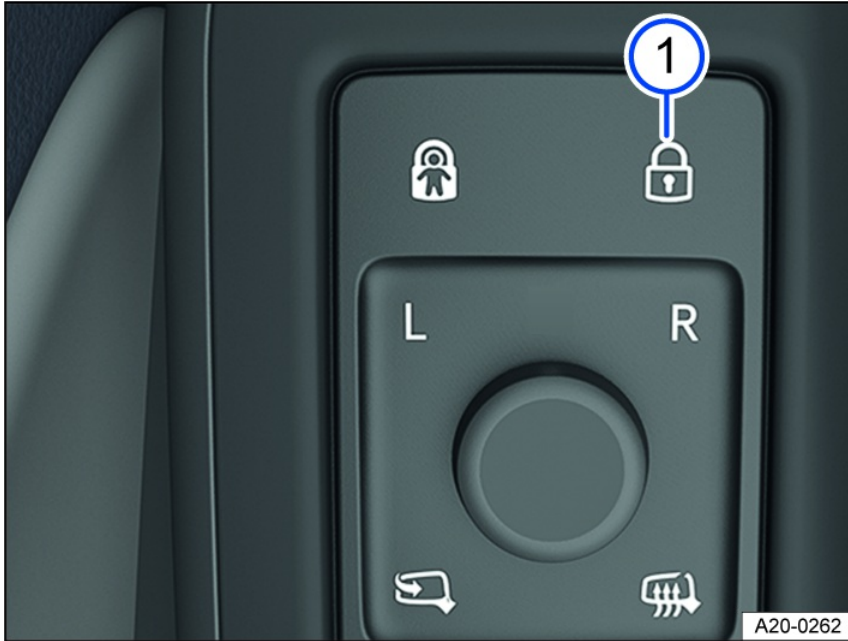
Fig. 45 In the driver door: Control for central locking.
