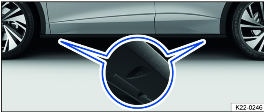
Fig. 171 Mounting points for the vehicle jack.
