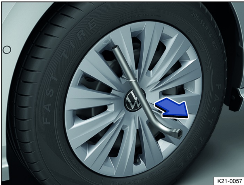
Fig. 168 Remove the wheel hub cover.
