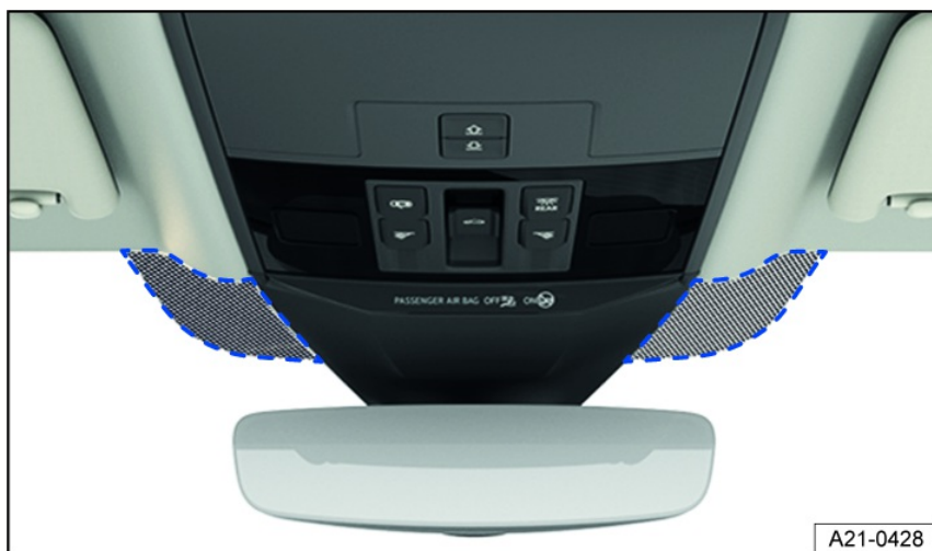
Fig. 82 Next to the mirror base: Communication window (general example).
