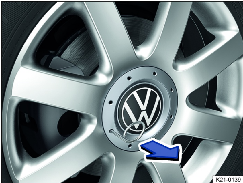
Fig. 167 Remove the hubcap.
