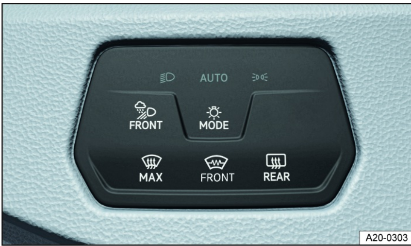
Fig. 72 Next to the steering wheel: Button to switch on the exterior lighting.
