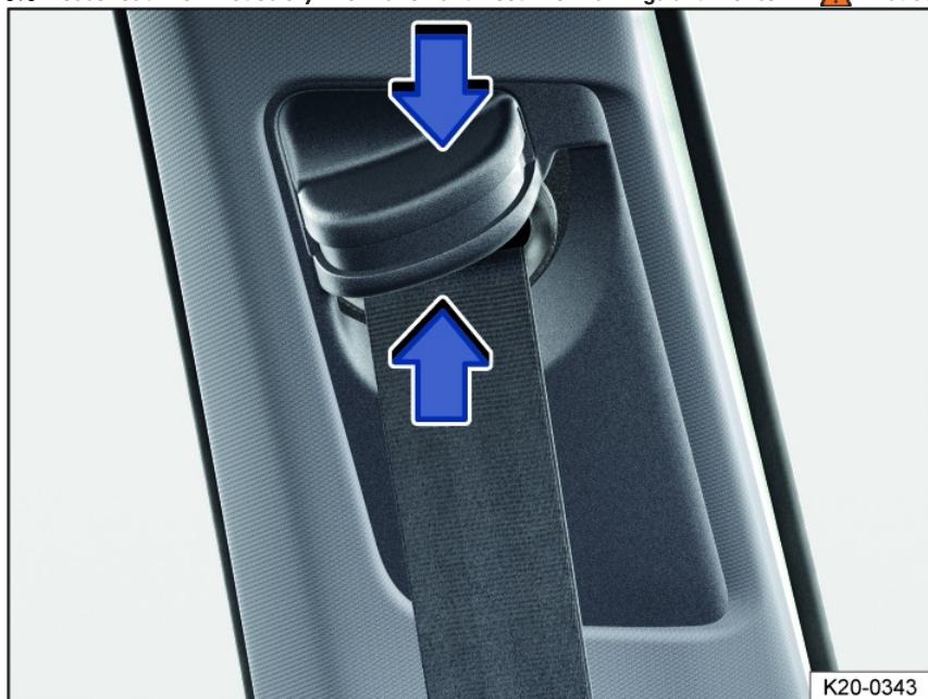
Fig. 20 Next to the front seats: safety belt height adjuster.
