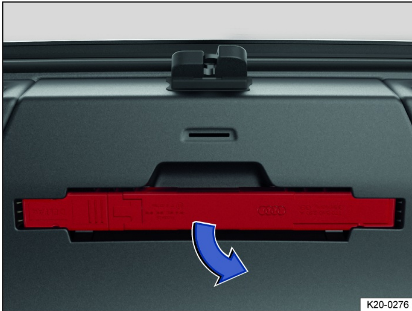
Fig. 35 In the trunk lid: Holder for the warning triangle.
