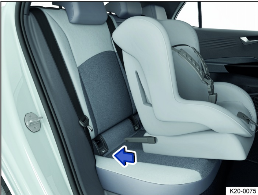
Fig. 30 General example: fitting a child restraint with attachment arms.
