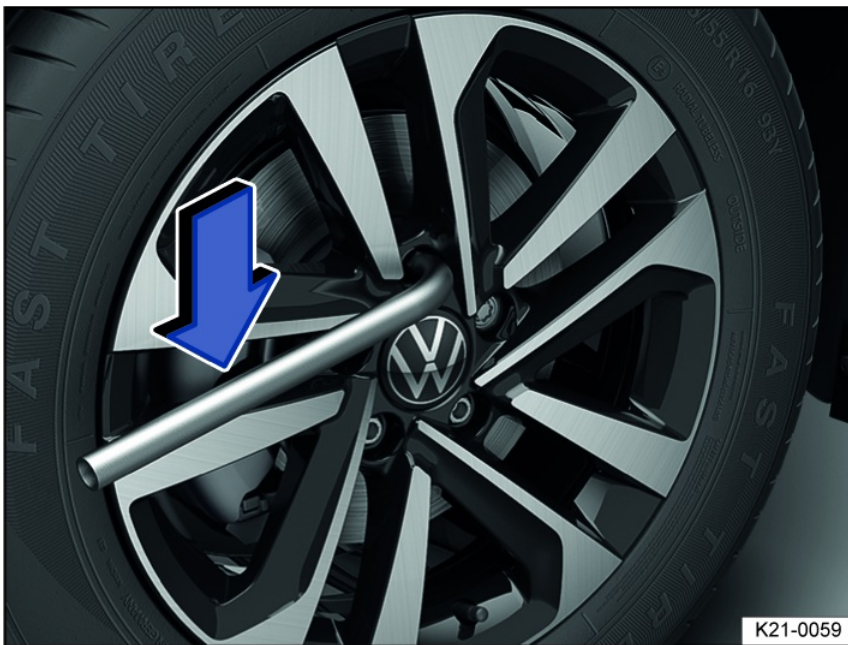
Fig. 174 Wheel change: removing wheel bolts with the lug wrench.
