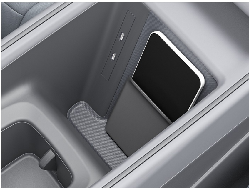
Fig. 111 General example: storage compartment with a holder for wireless charging in the center console.
