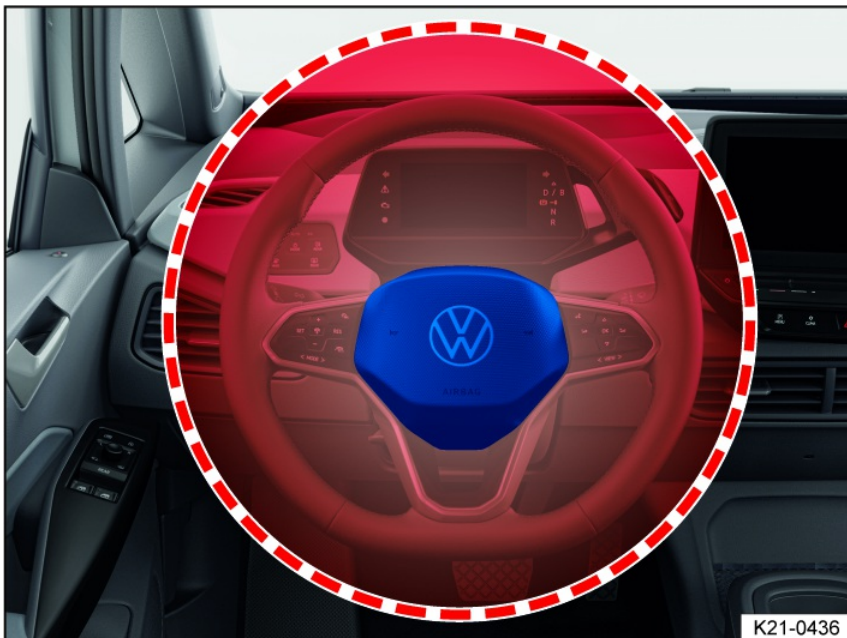
Fig. 23 Installation location and deployment zone of the driver's front airbag.
