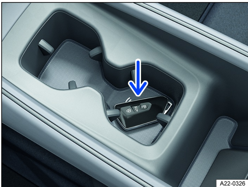
Fig. 84 In the center armrest: Emergency start function.
