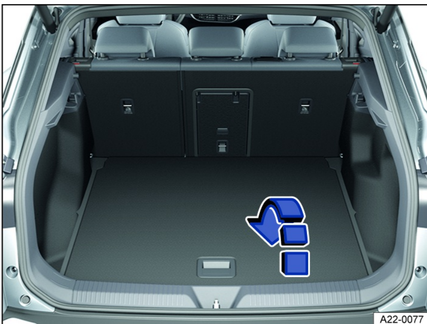
Fig. 117 In the luggage compartment: Opening the second luggage compartment floor.
