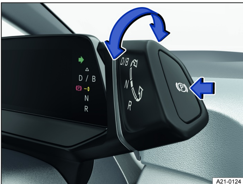
Fig. 85 Driving mode selector with the button for the electronic parking brake (arrow).
