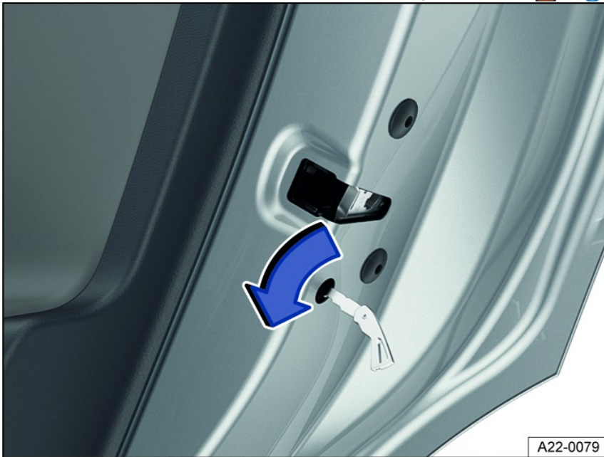
Fig. 48 In the front edge of the rear right-hand door: vehicle emergency lock for using the emergency key (general example).
