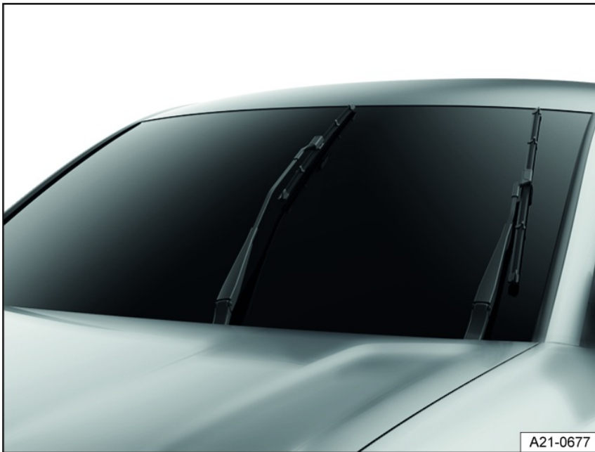
Fig. 141 Windshield wipers in service position (general example).
