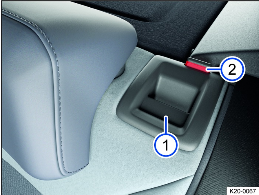
Fig. 62 In the rear seat backrest: release button.
