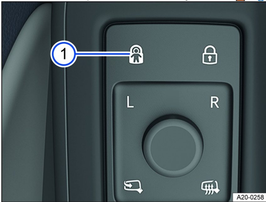
Fig. 49 In the driver door: Control for the electric child safety lock.
