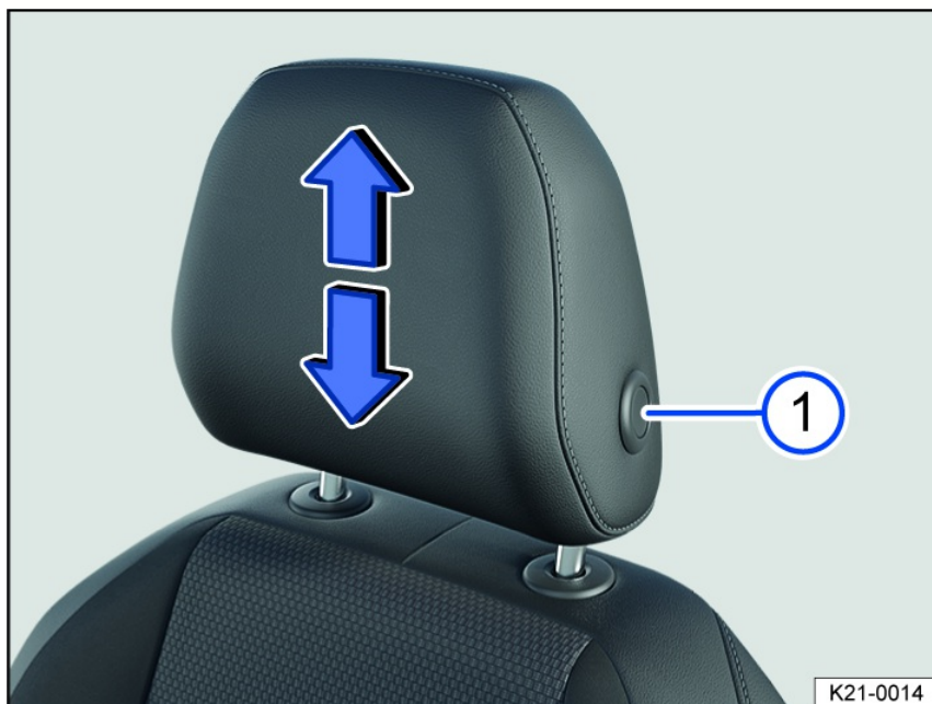
Fig. 63 Adjusting the front head restraint (general example).
