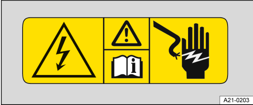
Fig. 126 Warning sign in the hood space.
