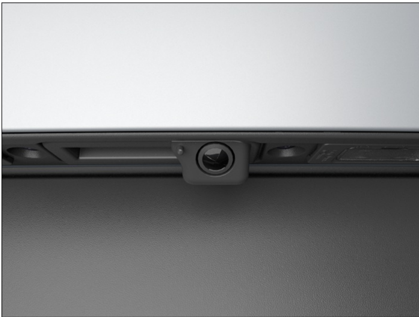
Fig. 180 In the rear of the vehicle: Rear View Camera system on the handle (general example).
