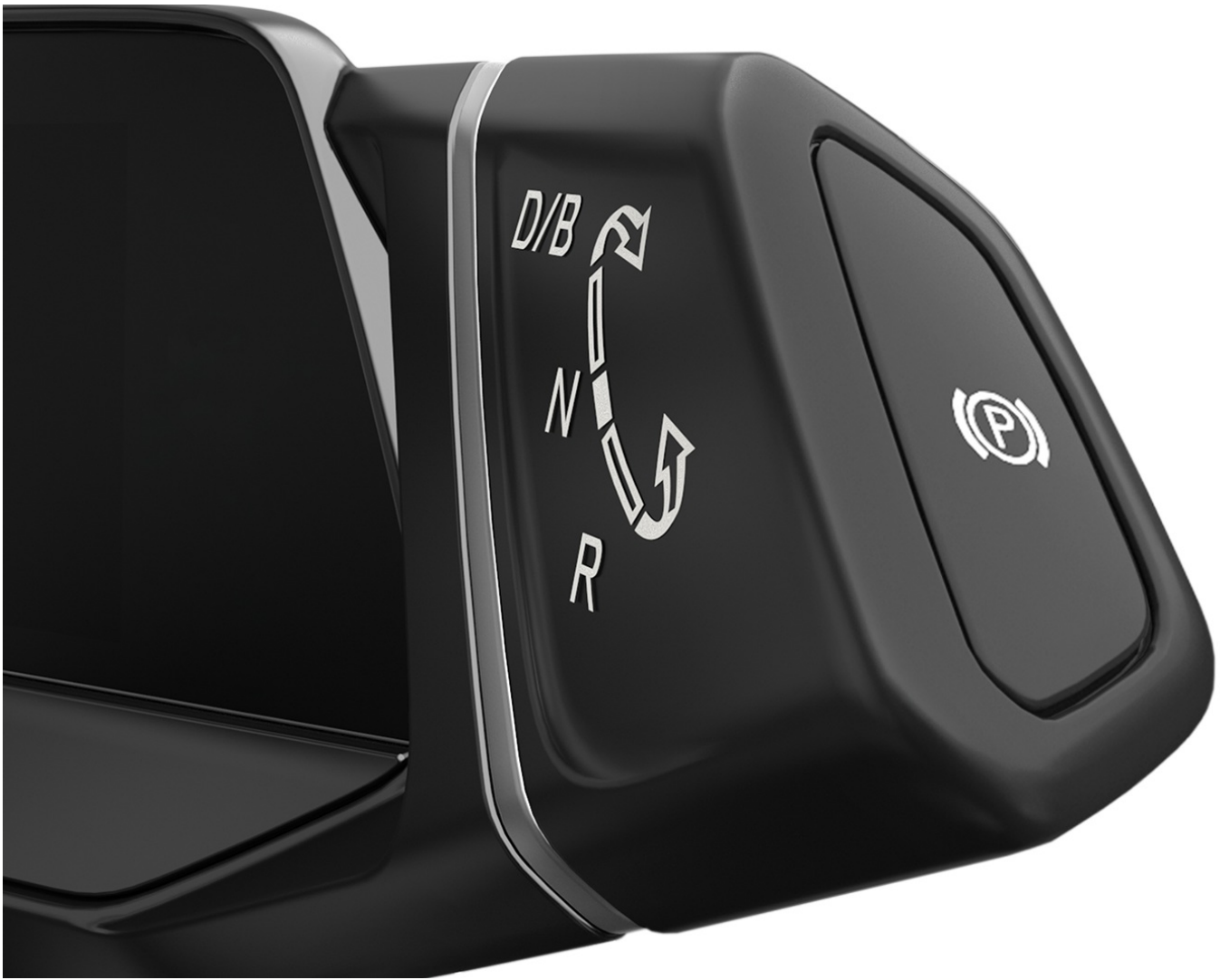
Fig. 98 On the driving mode selector: Button (P) for the electronic parking brake (general example).
