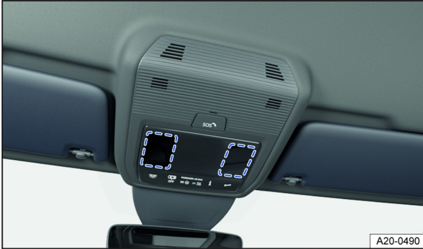
Fig. 74 On the overhead console: touch-sensitive reading lights.
