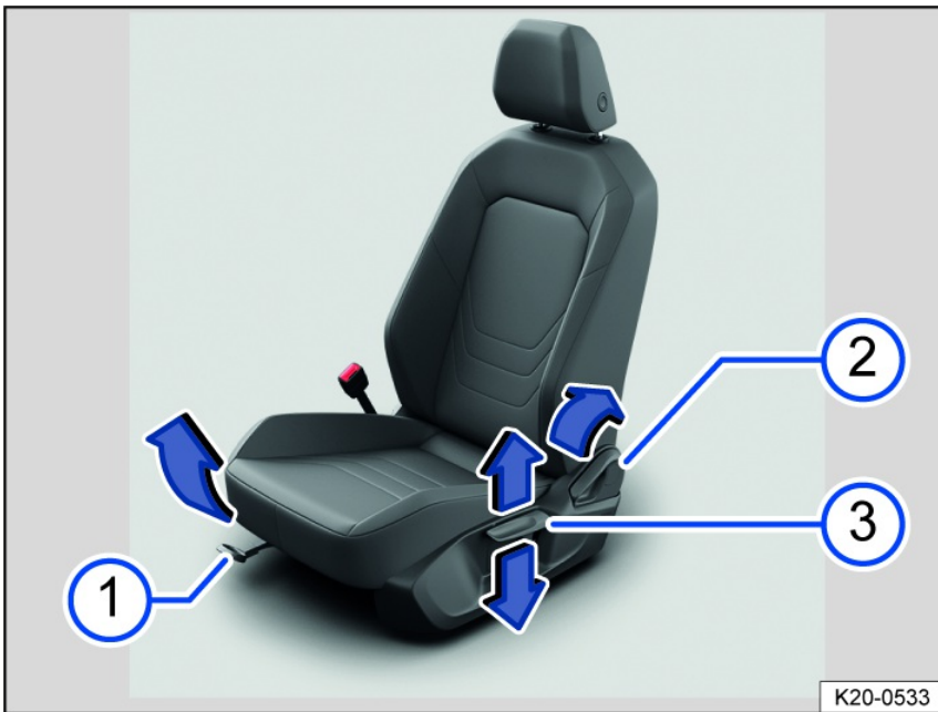
Fig. 59 On the driver seat: Controls.
