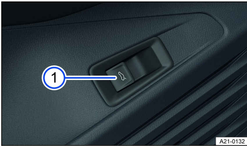
Fig. 52 In the driver's door: unlock button for the trunk lid.
