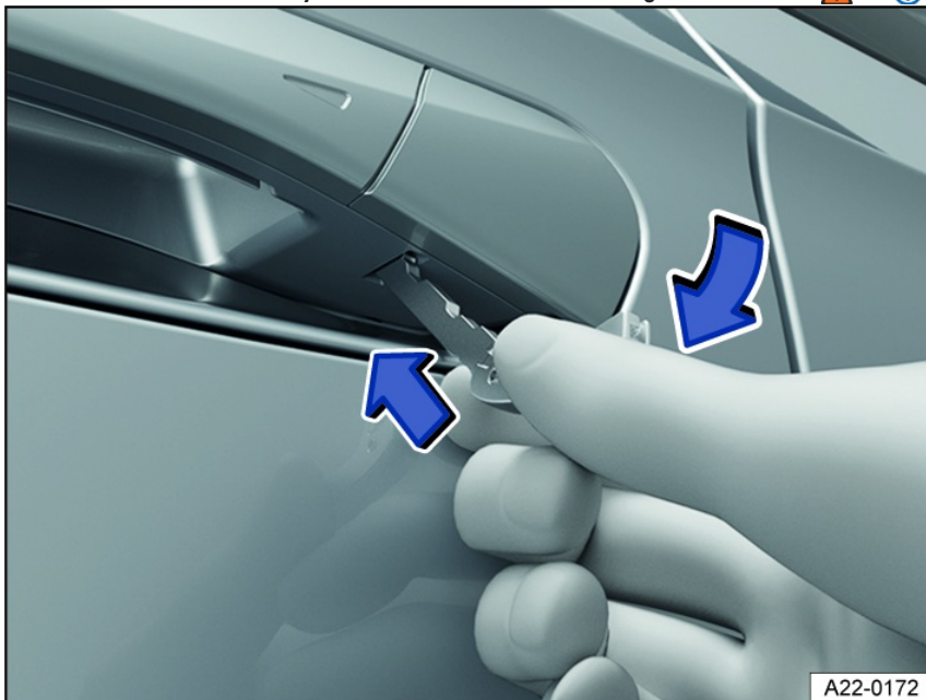
Fig. 46 Driver's door handle: prying off the cap.
