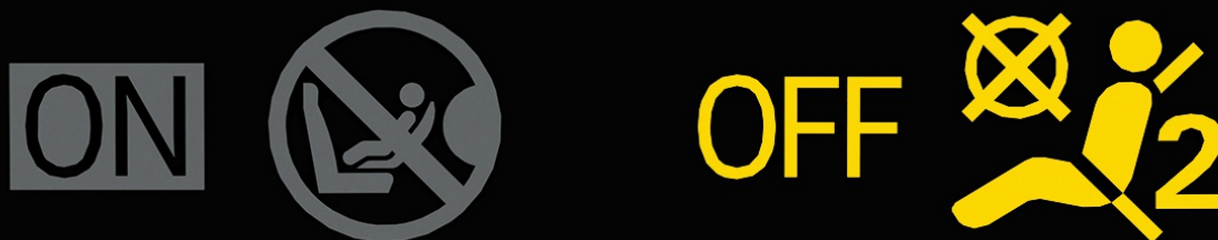
Fig. 21 In the roof console: indicator light (general example) for the switched off front passenger's front airbag.
