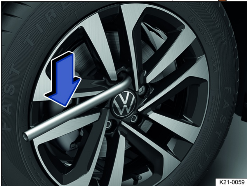
Fig. 170 Changing a tire: loosening the wheel bolts.
