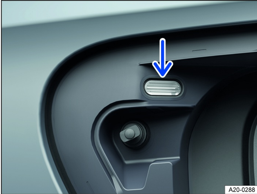
Fig. 131 Behind the charging socket flap: charging process indicator.
